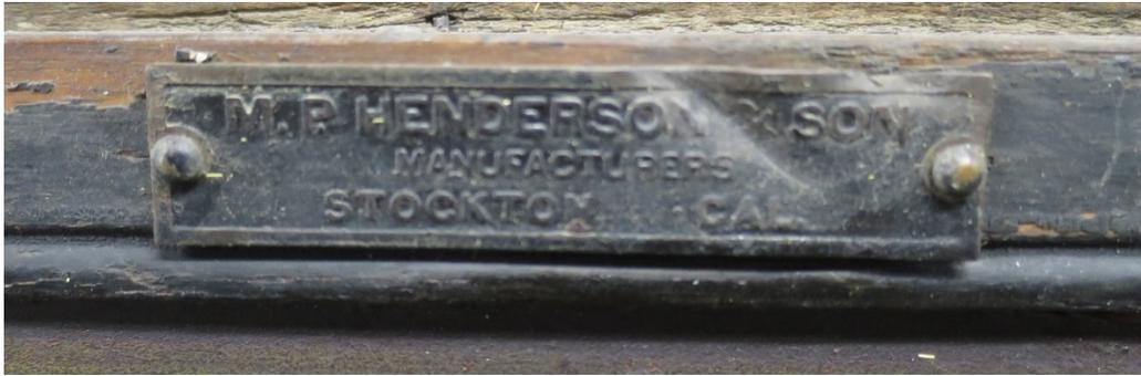
Is the tag original? It seems to be either cast or stamped into the plate and to have the patina that would suggest it is original. As the wagon was rolled at some time in its career, and the front boot mostly replaced, top supports sistered with steel strap and the thoroughbraces either repaired or built quite differently from the typical Henderson look bring some suspicion. There were also extensive non-conforming repairs to the thoroughbraces.
